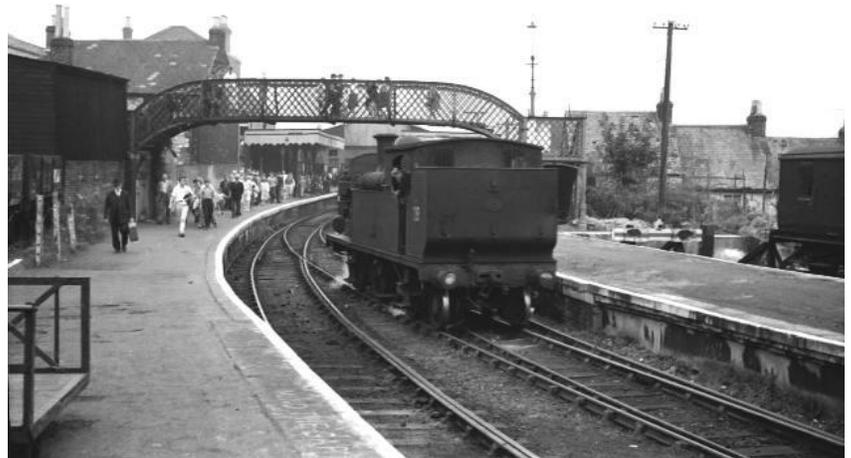
Arrived at Cowes, we watched as the engine completed its unusual run round manoeuvre, involving letting the coaches run down to the buffer stops under gravity controlled only by the Guard's handbrake, a somewhat hair raising procedure when encountered for the first time.
