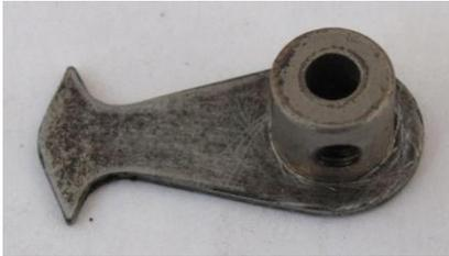
12) Pawl, part no. 33 (later part 147). This item was current only from 1921-25 and is now rare. It was incorrectly painted in dark green, but is now restored to nickel-plate finish. The shape was changed in 1925 to the more familiar pattern, and the part renumbered.
