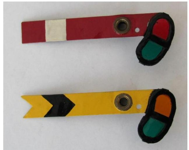
On restoration, red paint was found underneath the yellow, but with a straight white band on the front. Also, the end V notch appears to have been cut by hand, rather than machine. Thus the part has been modified at some time from a Home signal part 158a; rather thoroughly it seems, since the celluloid was also changed from red to amber!
