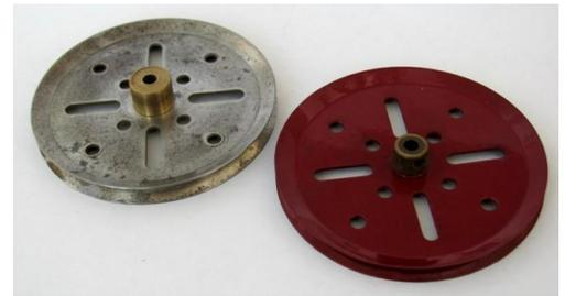
3) Pulley 1" diameter with boss, part no. 22. The standard 3/8" boss was introduced in 1913 (in place of keyways), but had only one tapped screw hole until March 1927 (this applies to all types of wheel and gears). Afterwards two tapped holes were provided, so this is a useful means of dating these items.
