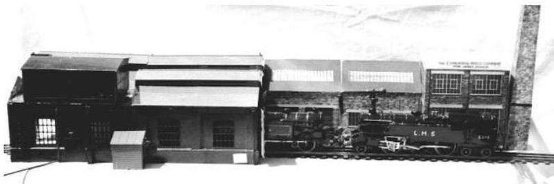
In comparison, the BR 2-6-4 tank loco escaped relatively unscathed, new plastic tank-side overlays being fitted to create an LMS-black liveried Fairburn version, numbered 2245, remaining as such to this day. Carefully filed-down side rods improved the appearance no end, on all the locomotives. The 2-6-4T is shown here in company with the “L&NWR” tank.....
