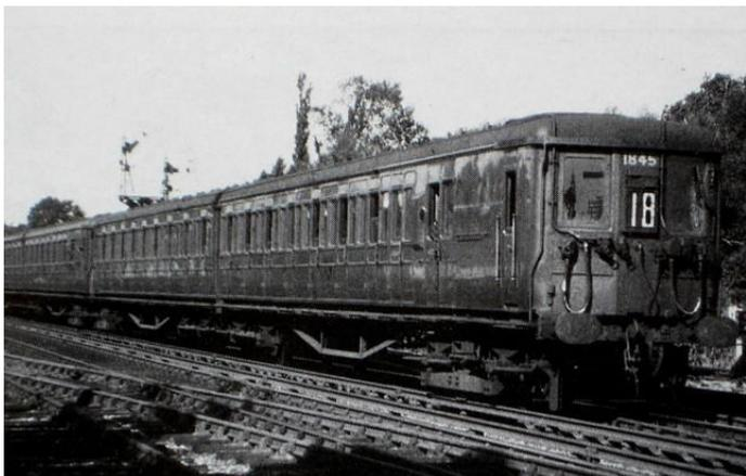
4-EPB ("electro pneumatic brake", thus breaking the traditional association with lavatories), and were common on our line from May 1957 onwards.
